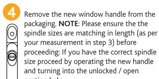
Remove the new window handle from the packaging. **NOTE:** Please ensure the the spindle sizes are matching in length (as per your measurement in step 3) before proceeding: If you have the correct spindle size proceed by operating the new handle and turning into the unlocked / open position below.
