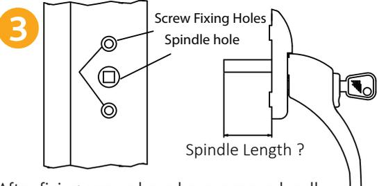
After fixing screws have been removed, pull to remove the handle from the window mechanism. This should reveal the two screw fixing holes and the square spindle hole. At this point please take note of the length of the current spindle size as shown above (?).
