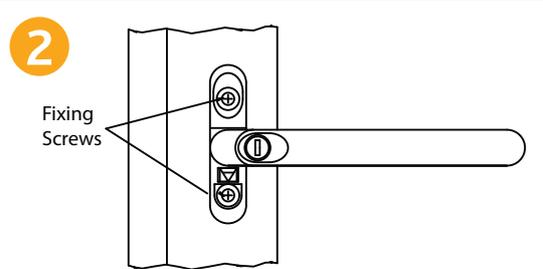
Remove both the top and bottom screw cover caps to reveal the fixing screw underneath. Using the correct screwdriver, remove both fixing screws
