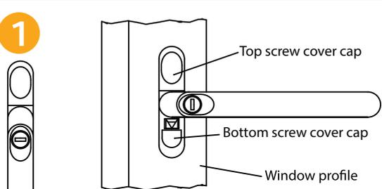
To remove the existing handle: If locked, unlock the window handle and turn 90° into the unlocked / open position as shown above. This should reveal both the top and bottom screw cover caps if present.
