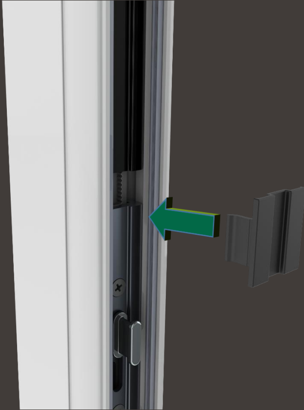
Step 7 Insert Facia Clip Covers between the Centre Lock and the Channel Covers , top and bottom
